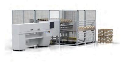
Electr. connection: 400 V / 50 Hz / 3 phases Power supply: 16 A/phase Efficiency: motor IE3 - class Pneumatic supply: 5.5 bar Air consumption: 1.7 m<sup>3</sup>/h
