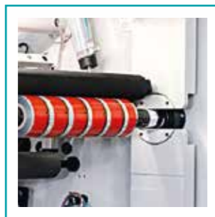
8 Reel pushing system from top: safe and clean rack and linear guides
