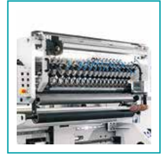
6 Additional comfort kit to improve the accessibility to the slitting section, while maintaining a compact configuration
