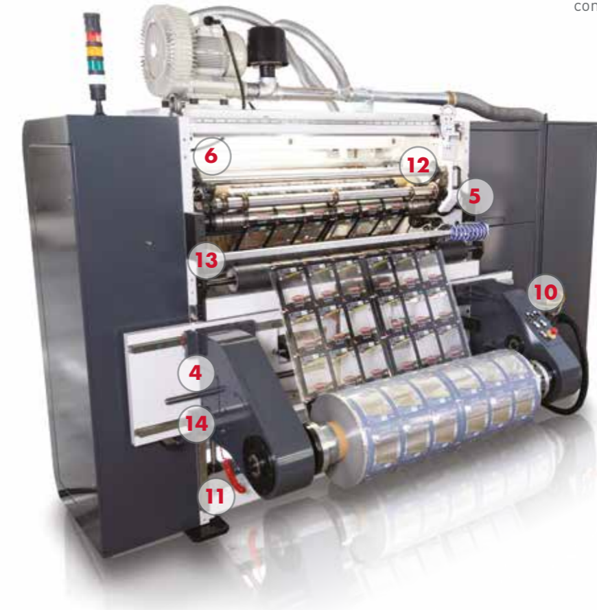
5 Blade oscillation function for razors slitting
