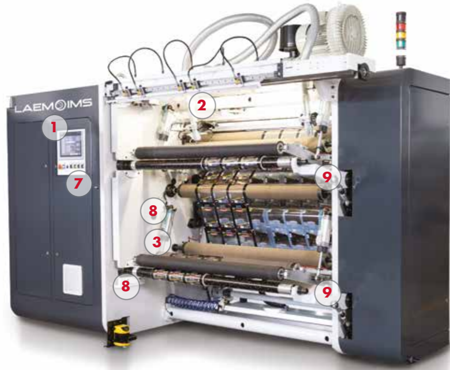
1 User-friendly HMI with push buttons, featuring a pivoting console that houses a Siemens color operator touch panel to perform the main machine functions
