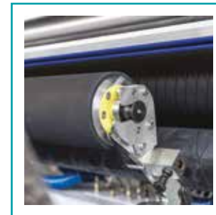
8 Easy and "quick change" contact rollers, no tools needed
