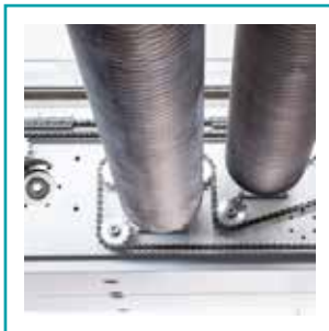
5 S-roller group with high wrap-around angle for optimal web tension separation
