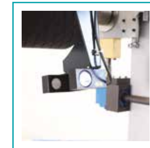
10 Web edge guiding with optional oscillating function
