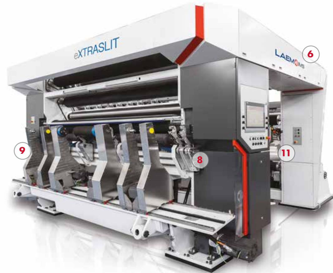
4 Guide rollers with different coatings available. Driven dancer roller, chrome-plated rollers and individually driven rollers are available for delicate materials
