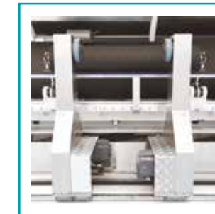
9 2000 kg, 3300 kg and 5000 kg rewind stations available with manual or fully-automatic positioning
