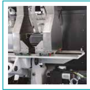
2 Loading and unloading reels movements are electrically driven
